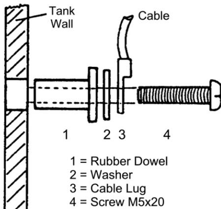
**Fig. 4: Conductor with Metal Tanks**
