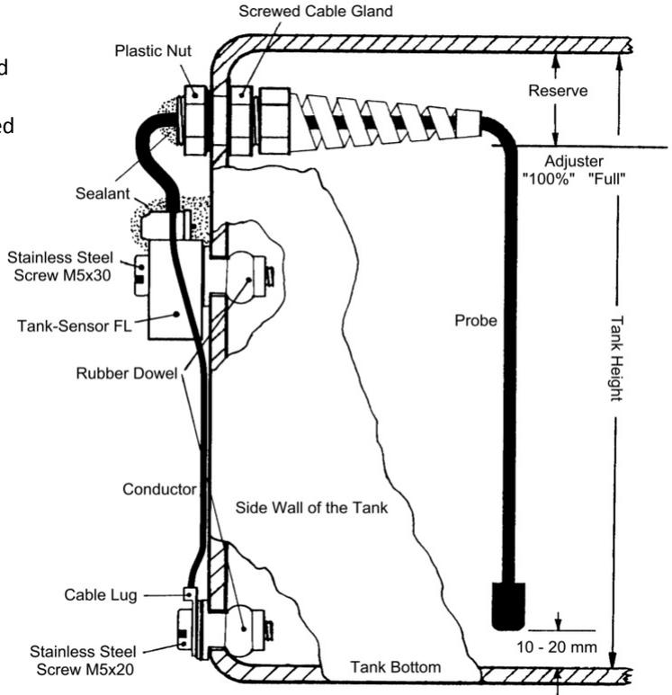
**Fig. 3: Conductor with Plastic Tanks**
