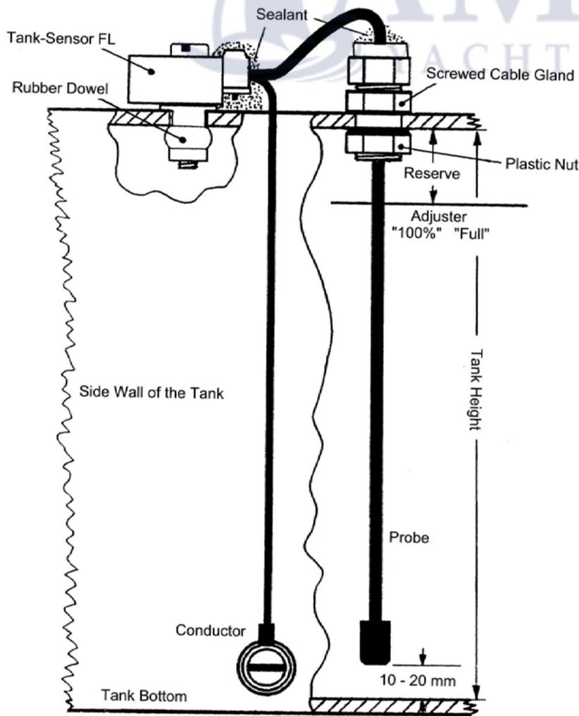
The fill level in the tank is measured capacitively. This is because the probe forms with the surrounding water a "capacitor" whose value increases with the fill level measured by the Tank Sensor FL. The compound to the water as an "antipole" is formed by the "conductor".
